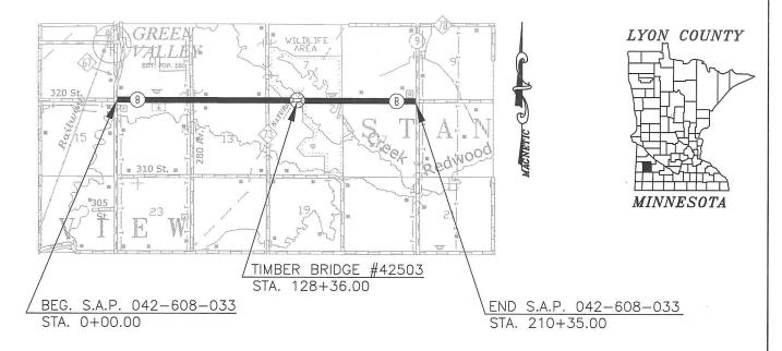
FUNCTIONAL CLASSIFICATION: MINOR COLLECTOR POSTED SPEED: 50 MPH ADT (2025): 160 PROJ ADT (2045): 176 NO. OF TRAFFIC LANES: 2 S.F. 130 % R VALUE:10 TON DESIGN:10 ESALS (20 YR):53,000 SHOULDER WIDTH: 4' STOPPING SITE DISTANCE BASED ON: 3.5' HEIGHT OF EYE 2.0' HEIGHT OF OBJECT GRADED: 042-608-04 (1960) SURFACED: 042-608-26 (2001)
