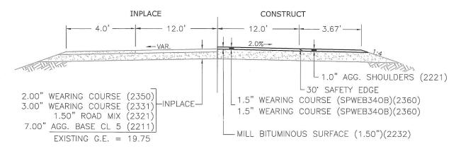
GRANULAR EQUIVALENT 10 TON R VALUE: 10 ESAL'S: 53,000 (20 YR-FLEX) REQUIRED G.E. 16.00 G.E. ON PLANS: 26.50
