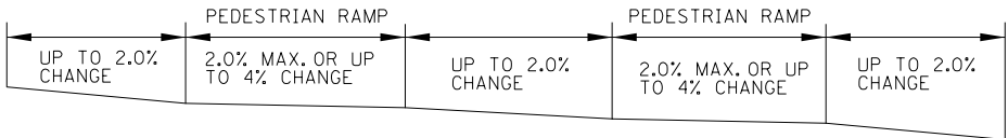
FLOW LINE PROFILE "TABLE" - TWIN PERPENDICULARS
