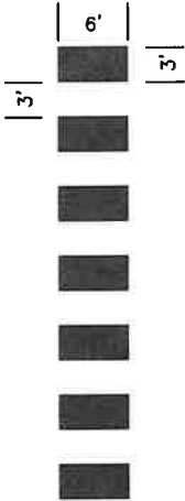
TYPICAL CROSSWALK STA 28+93, 31+99 AND 34+24
