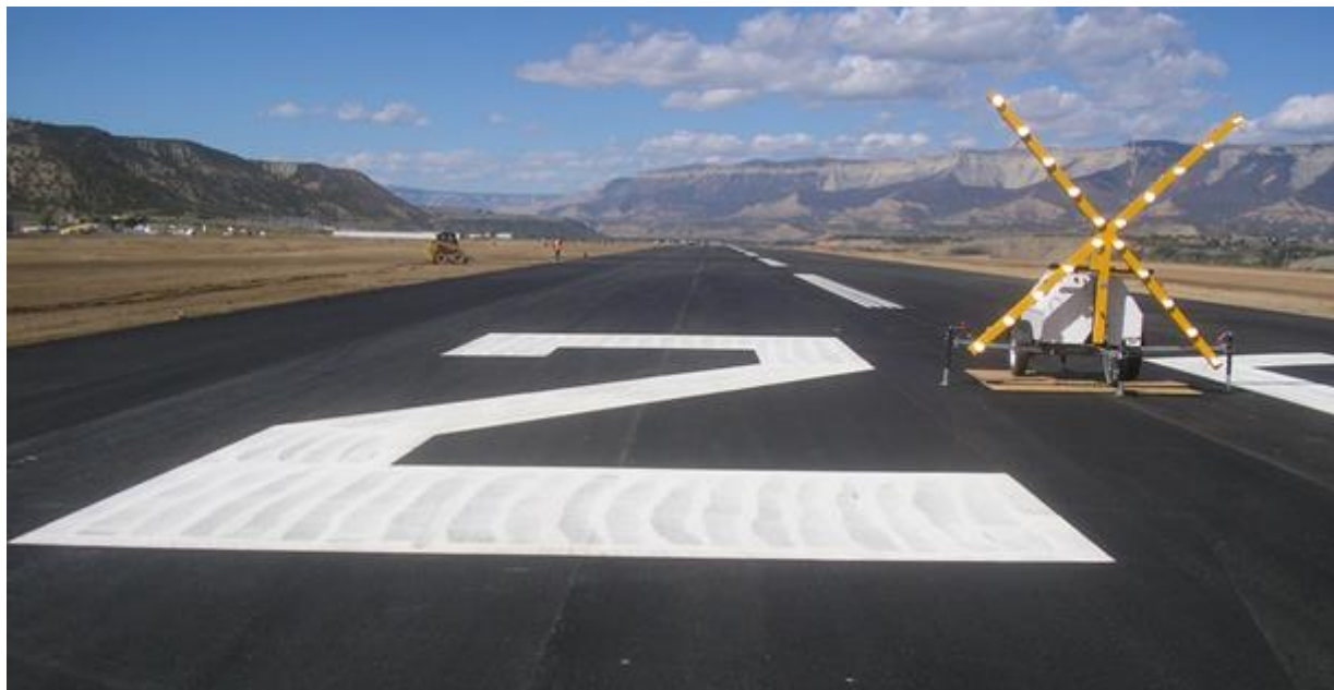
Figure 2-7. Lighted X at Night
