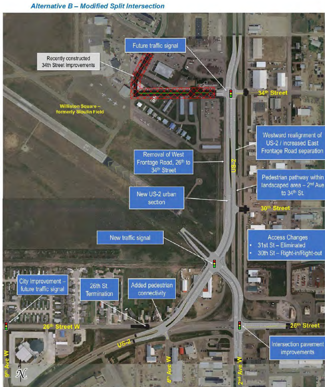
Figure 4: Alternative B – Modified Split Intersection
